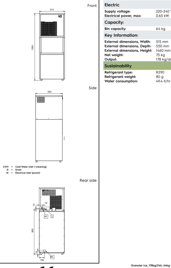
Ice Makers Granular Ice, 178kg/24h, 64kg bin, water-cooled
